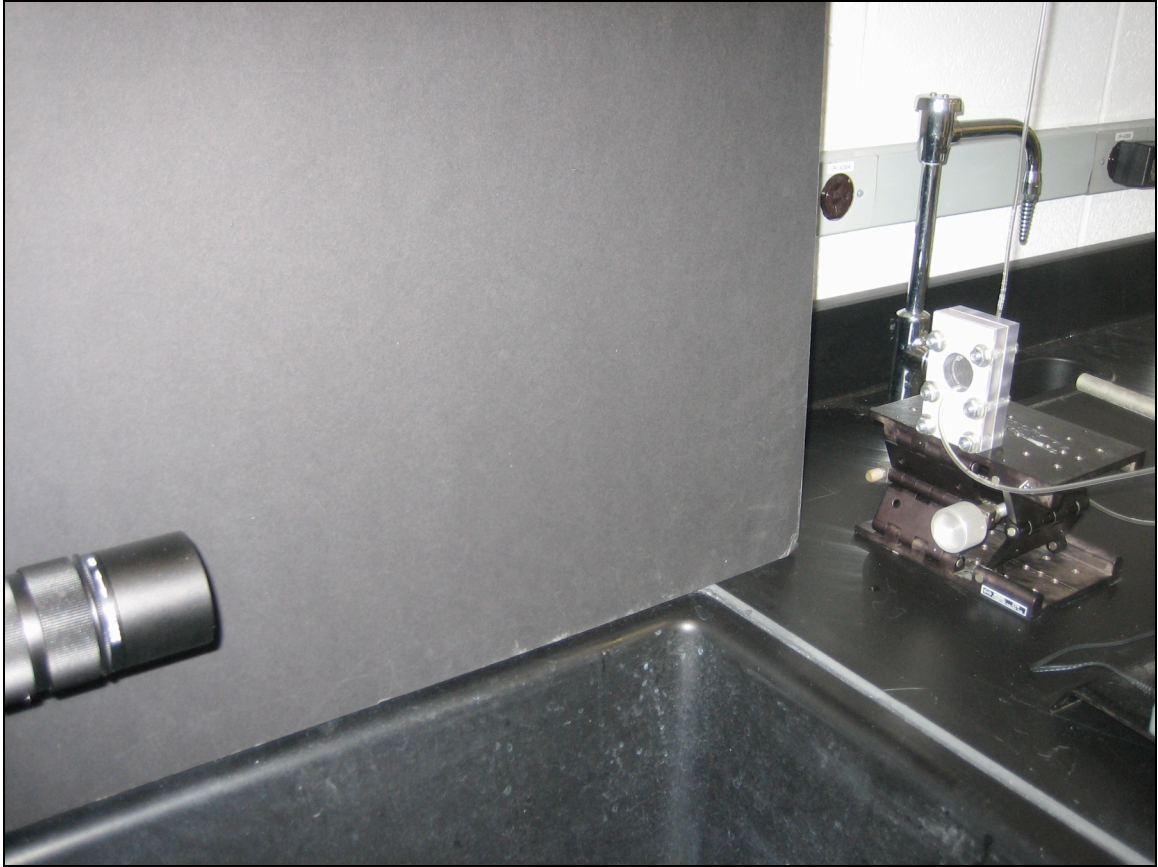
Figure 7. The camera was positioned to capture water droplet formation and detachment on the "gas side" of the membrane.
