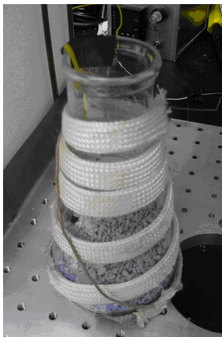
Figure 3.3: Water desorption environment containing drierite. Heating tape controlled the interior temperature.
