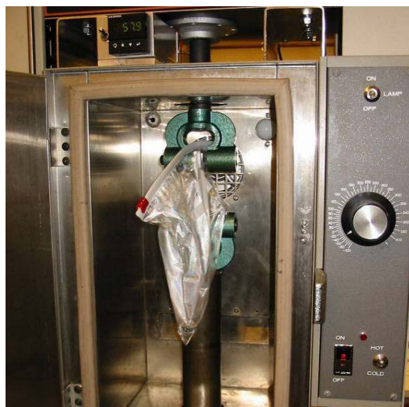
Figure 2.13: Instron 1122 outfitted with plastic bag vapor barrier for elevated humidity tests.
