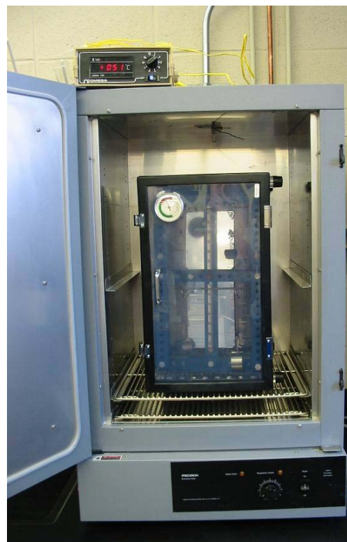
Figure 2.15: Controlled humidity & temperature creep experiment
