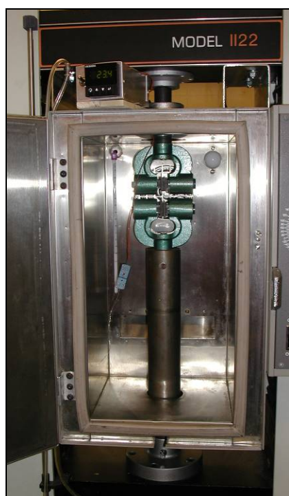
Figure 2.12: Instron 1122 & environmental chamber used for stress-strain tests
