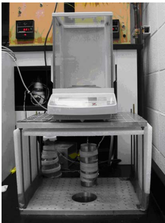
Figure 3.1: Water Sorption Set-up: Membrane hung from a bottom-weighing scale into the controlled-atmosphere chamber and weight was continuously recorded. Figure reprinted from 17 with permission from Elsevier © 2007. Image has been cropped & text box removed.
