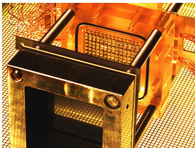
Fig. 1. Photograph of segmented anode flow field showing current-collectors and optical and infra-red viewing window.
